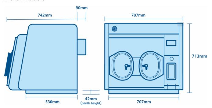
**Important note:** In addition to the dimensions stated above (non-HEPA model), allow a localised protrusion of 90mm at rear to accommodate condenser bottle, bracket, gas and electrical supplies. If bench mounted, a further minimum clearance of 500mm is required above the unit and a minimum clearance of 500mm at the right-hand side of the unit is required for user/service access.
